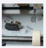
• Initial transversal cut before profiling : allows profiling direct from a roll starting with a straight cut.
