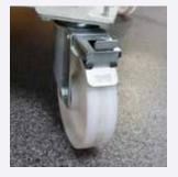
• The wheels fitted with brakes avoids the risk of the machine moving during use or transport.
